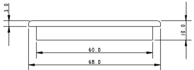
**Details:** CNC machined in-house. The A8040-56 has rope friendly radiused edges and a modern look. Perfect for bonding into a deck to allow a tidy pass through for control lines. Anodised dark grey.
