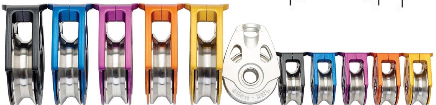
**Details:** The A2020XHL has been designed to deal with extremely high loads without compromising on low load dynamic performance. By combining our patented dynamic bearing technology with CNC machined aluminium side cheeks and a precision turned stainless steel sheave, we have created a block that can take a static load of 900Kg. Perfect for use in vang cascades or halyard turning points where loads can be extremely high.
