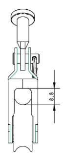
Details: The A2030F-873 features an adapted side strap for a clevis pin attachment. This block also comes with a strengthened vang key. 30mm Dynamic Blocks use the same high quality Dynamic bearing, materials and precision engineering as our 20mm Dynamic Block range.
