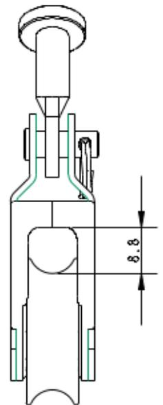
**Details:** The A2030F-873 features an adapted side strap for a clevis pin attachment. This block also comes with a strengthened vang key. 30mm Dynamic Blocks use the same high quality Dynamic bearing, materials and precision engineering as our 20mm Dynamic Block range.
