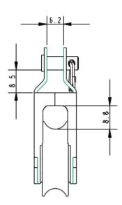
Details: The A2030F features a fork head with removable clevis pin making it a customisable block to multiple applications. This 30mm Dynamic Blocks use the same high quality Dynamic bearing, materials and precision engineering as our 20mm Dynamic Block range. The block also features a central rivet that provides great options as a tie on becket.
