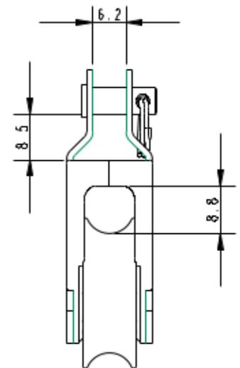
**Details:** The A2030F features a fork head with removable clevis pin making it a customisable block to multiple applications. This 30mm Dynamic Blocks use the same high quality Dynamic bearing, materials and precision engineering as our 20mm Dynamic Block range. The block also features a central rivet that provides great options as a tie on becket.
