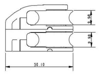
Details: The A2136M features the same dynamic bearing technology you will find in the rest of the 30mm dynamic block range; two rows of 316 stainless steel ball bearings located around a central axle. The A2136M also has two fixing holes and an inter-locking middle cheek face to ensure that there is no movement once fixed to the deck and put under load.
