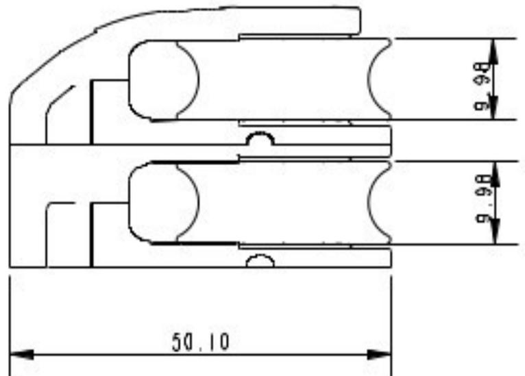
**Details:** The A2136M features the same dynamic bearing technology you will find in the rest of the 30mm dynamic block range; two rows of 316 stainless steel ball bearings located around a central axle. The A2136M also has two fixing holes and an inter-locking middle cheek face to ensure that there is no movement once fixed to the deck and put under load.
