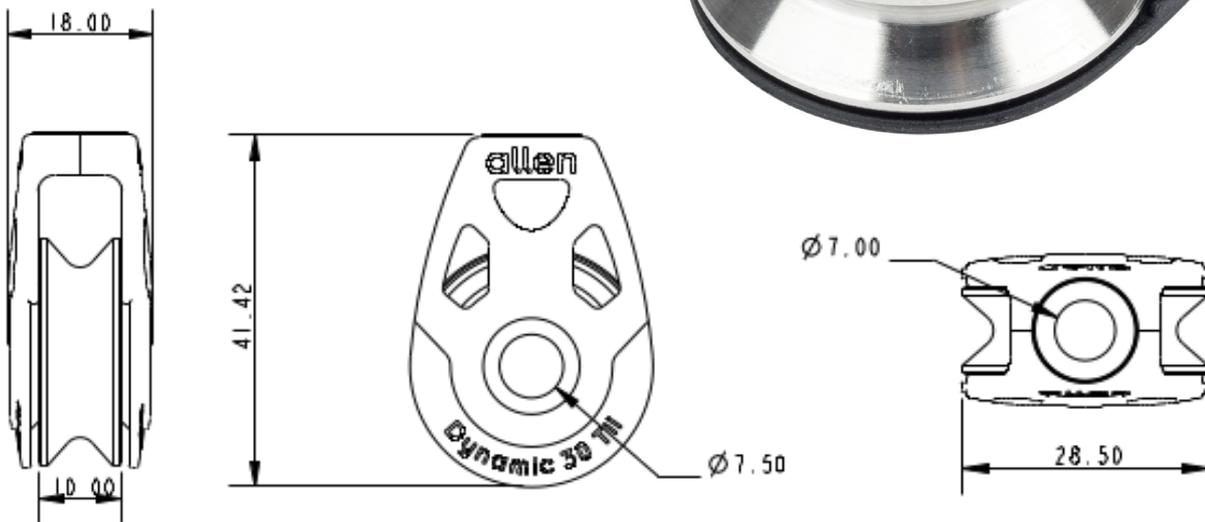
**Details:** This HL version of the A2030Tii also includes the high load sheave from our popular range of high load blocks. A stainless steel sheave running on our dynamic stainless steel bearings provides higher working loads and better performance compared to our standard acetal sheave range.
