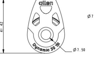
Details: This HL version of the A2030Tii also includes the high load sheave from our popular range of high load blocks. A stainless steel sheave running on our dynamic stainless steel bearings provides higher working loads and better performance compared to our standard acetal sheave range.
