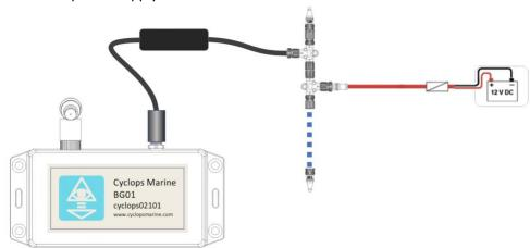
The sensor is now broadcasting load data to the gateway (and the instruments).
