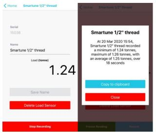
This button records the specific load data until 'Stop Recording' is pressed. A summary of the data is then displayed onscreen, with an option to copy the summary to clipboard for pasting into another app e.g. Notes
