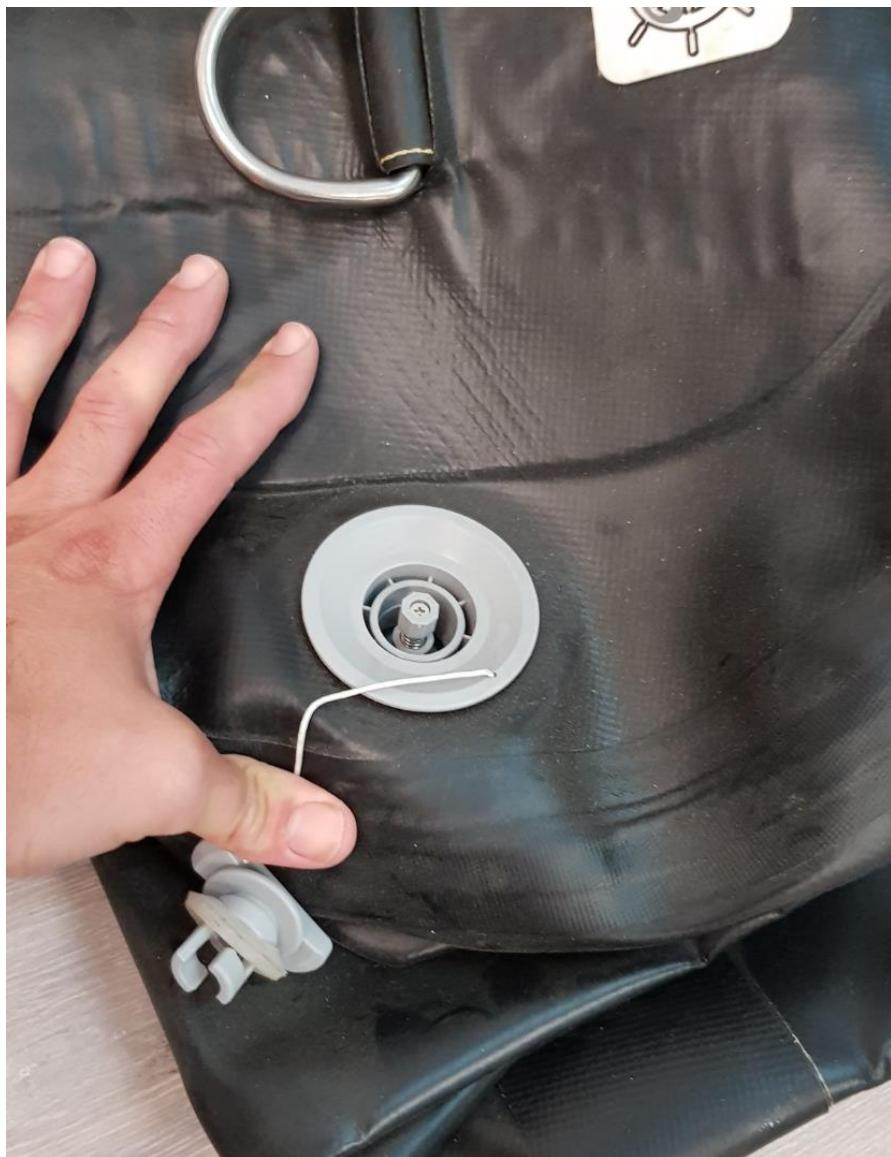
2- INSERT THE TOOL INTO THE VALVE AND ROTATE COUNTERCLOCKWISE TO REMOVE THE OLD VALVE
