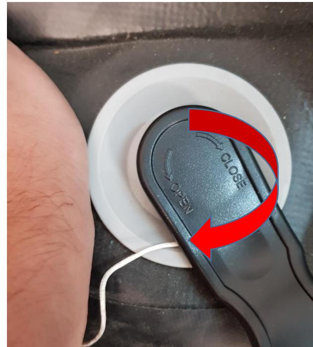
5- TIGHTEN THE VALVE BY USING THE TOOL PROVIDED
