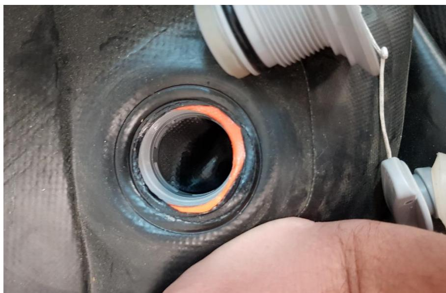
4- PUT THE NEW VALVE AND ROTATE CLOCKWISE
