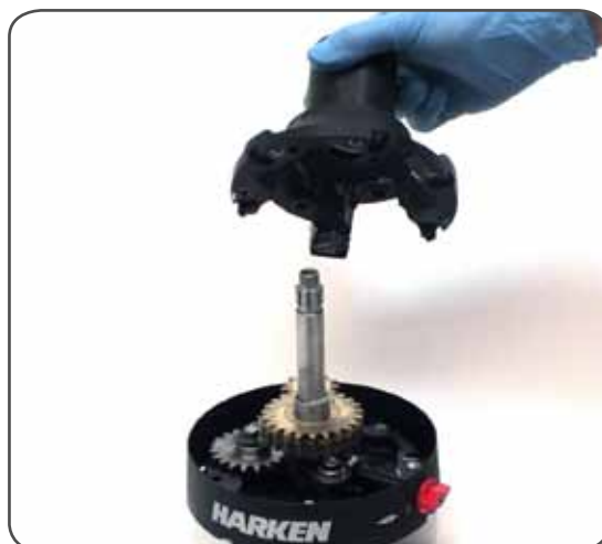
10. Remove drum support n°11
