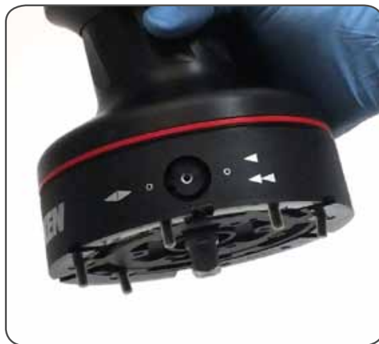
4. Reposition the skirt n°2 in its housing
