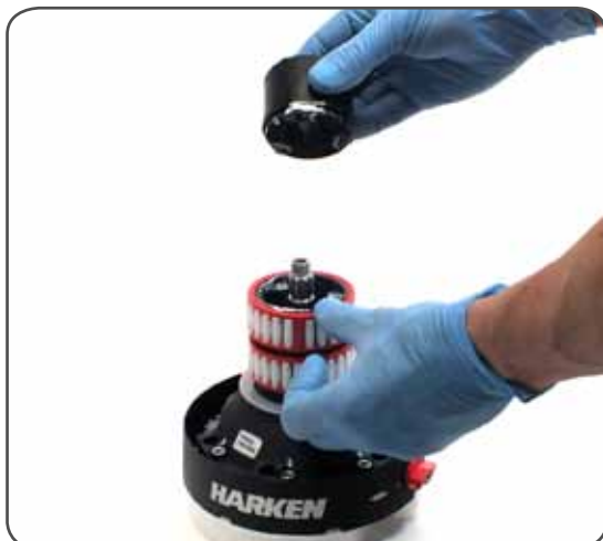
7. Remove the stripper arm support n°16
