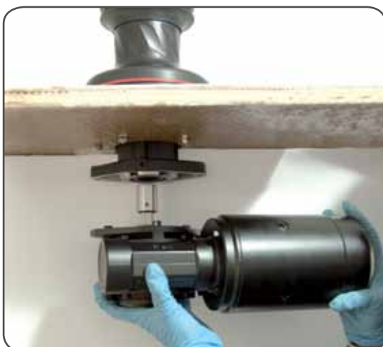
3. Position the reduction gear and motor
