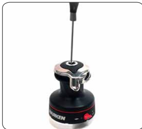
2. Unscrew the central screw ( \approx 2\text{Nm}/18\text{ in-lb} )
