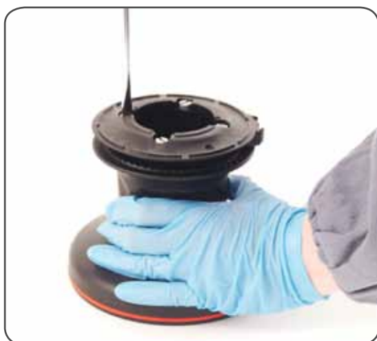
I. Unscrew the 4 screws n°18 (4Nm/35 in-lb)
