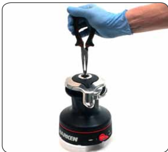
1. Pull out the disconnect rod n°31
