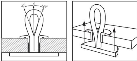
Ropeye Loop is designed for vertical loads with maximum loading angle of 20 degrees.
