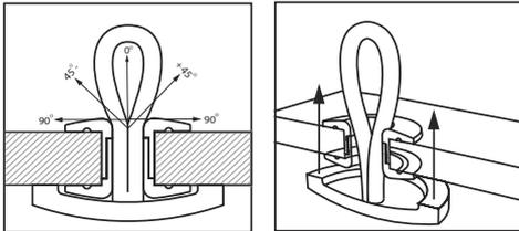
Ropeye PRO Loop is designed for loads in every direction without decreasing working load.
