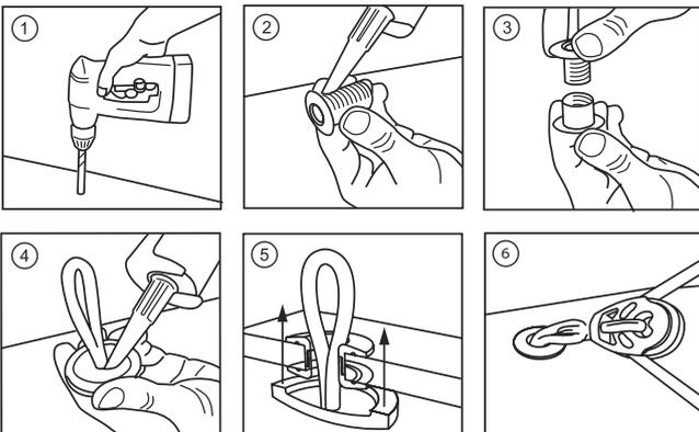
Drill a hole for the double TDP. Clean the installation area with acetone to remove dust and grease. Apply Sikaflex 291i or other adhesive to make the installation watertight. Tighten the double TDP. Attach the SLR to the loop. Wait 24 hours before putting any load on the product.
