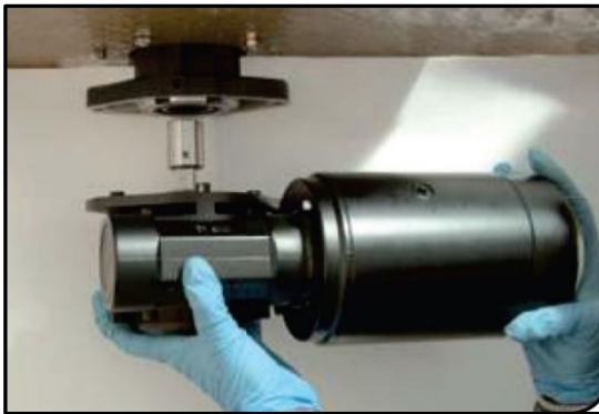
I. Position the reduction gear and motor
