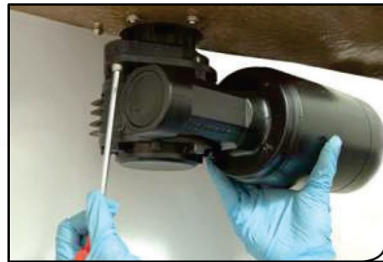
L. Tighten the two M6 precote screws (8Nm/71 in-lb) - be sure to align the flange
