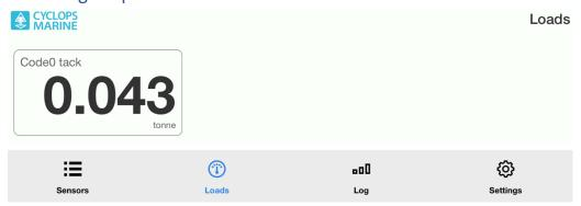
All sensors added on the 'Sensors' page will appear here. If a sensor is not powered on or in range, the last detected load value will show in grey.
