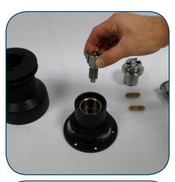
1. Planetary shaft must be centered in the center stem gears.
