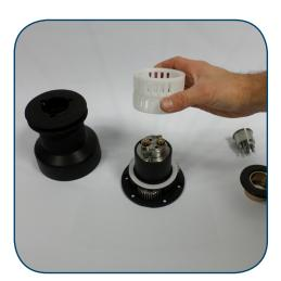
Rince Needle bearings with fresch sprayed water.
