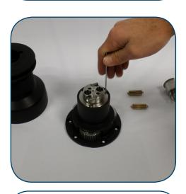
7. Remove the screws on compact pawls support
