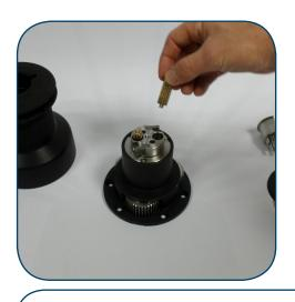
6. Remove feeder arm gear
