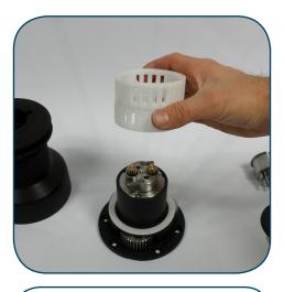
4. Remove the needles bearing
