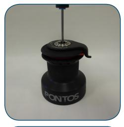
Unscrew the handle socket with Pontos Key and a screwdriver
