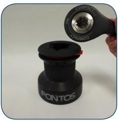
Remove the feeder arm et the handle socket
