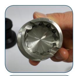
2. Rotate planetary shaft into the pawls support.
