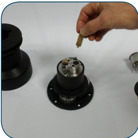
6. Remove feeder arm gear
