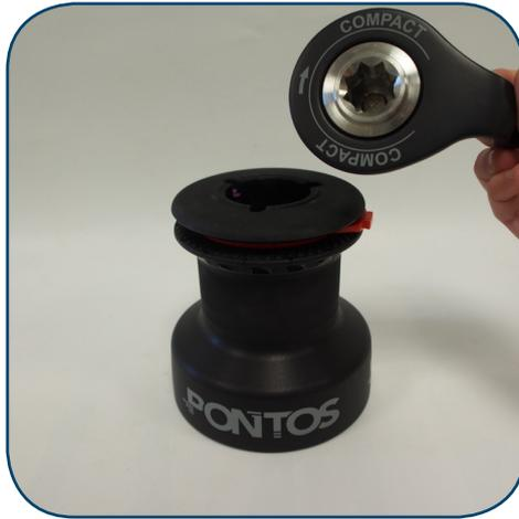
2. Remove the feeder arm et the handle socket
