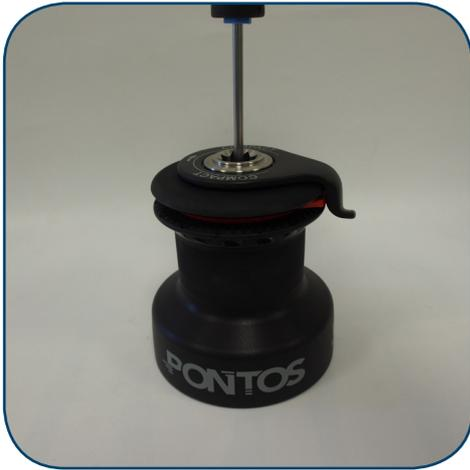
1. Unscrew the handle socket with Pontos Key and a screwdriver
