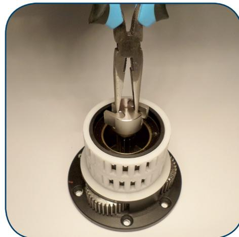
9. Extract the planetary shaft with a pair of long nose pliers
