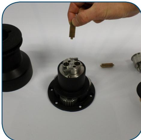
7. Remove the screws on compact pawls support
