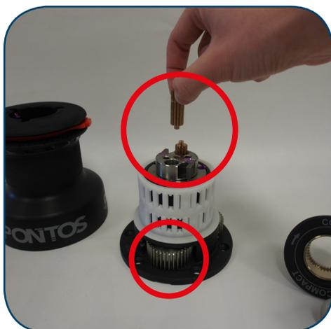
1. Clean all pinions and shafts. Add marine grease with moderation. Grease excess might retain salt.
