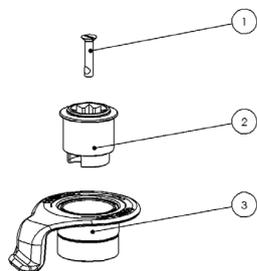
1. Remove the handle socket screw
