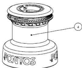
4. Lift and remove the drum.
