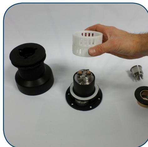
2. Rinse Needle bearings with fresh sprayed water. Never grease them !
