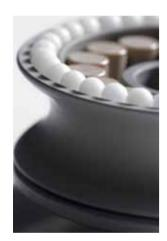
KBO bearing has been designed to enhance the free spinning of the sheave. KBO blocks feature two stage of bearing (Roller bearings for radial loads, ball bearings for axial loads). Thus, it ensures low friction even when the line is running through a tricky angle.
