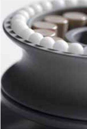
KBO bearing has been designed to enhance the free spinning of the sheave. KBO blocks feature two stage of bearing (Roller bearings for radial loads, ball bearings for axial loads). Thus, it ensures low friction even when the line is running through a tricky angle.
