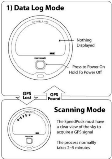
The data logger operation option is available in case rules prevent you from using the features offered by the SpeedPuck. The data logger mode displays blank, but records your GPS data which can be replayed later for analysis.
