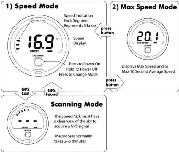
The motor sports operation option is for the motor sports enthusiasts who want to know exactly how fast they are going. No heading information is displayed in this operation as speed is the focus. The bar graph acts as a secondary speedometer in speed mode so you know how fast you are going at a glance.
