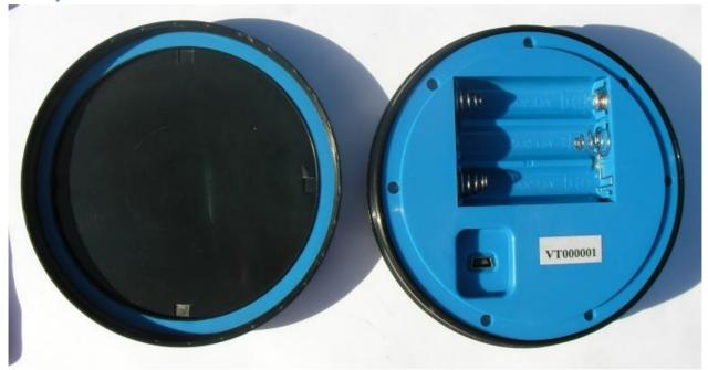
The SpeedPuck requires 3 AA batteries to operate. The battery compartment can be reached by opening the back case.
