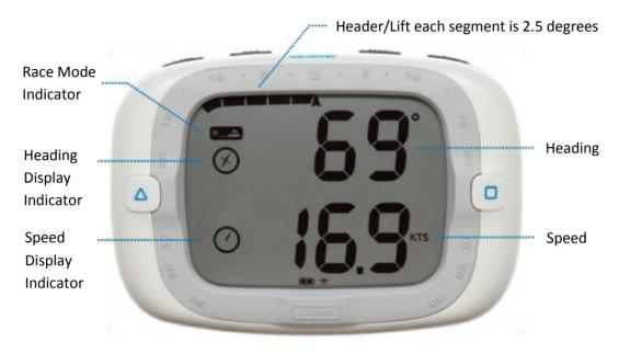
The race mode displays information crucial during the race, speed, heading and header/lift to the sailor.
