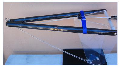
Fig 5: Showing flat nylon webbed Stop Strap.
