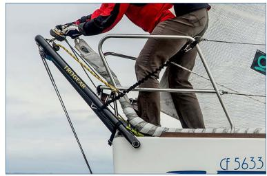
Fig 3: Bowsprit in upright position to attach a furler.
