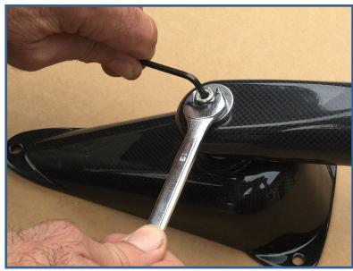
Fig. 2: Use allen wrench to prevent stud rotation
