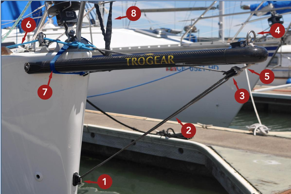
1. U Bolt (shown here with low friction ring)
