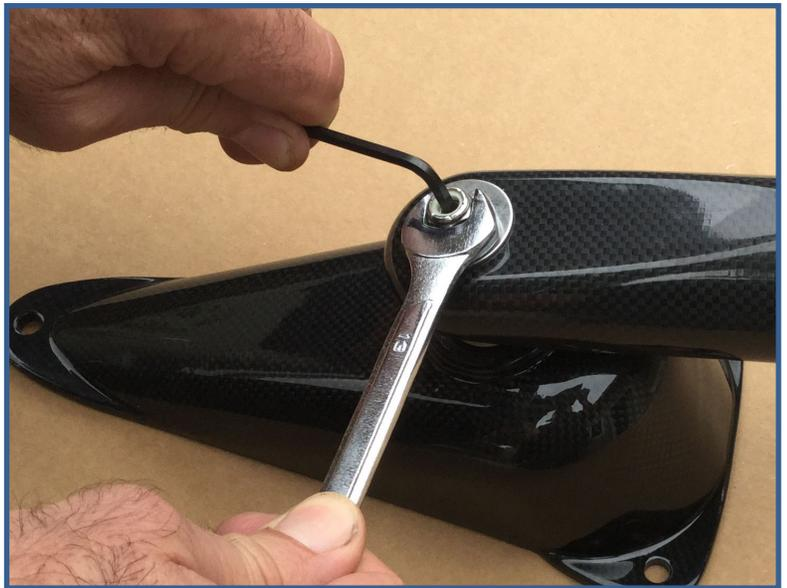
Fig. 2: Use allen wrench to prevent stud rotation
