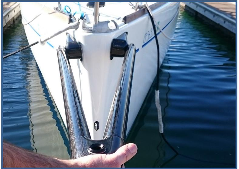
Fig. 1: Place bowsprit with mounts attached on the hull to determine location
