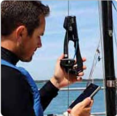
Rig Tension gauge for repeatable rig settings - aids race set up and preparation.
