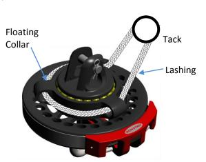
Pulling on this line while furling will keep the tack clear of the torsion cable.)
