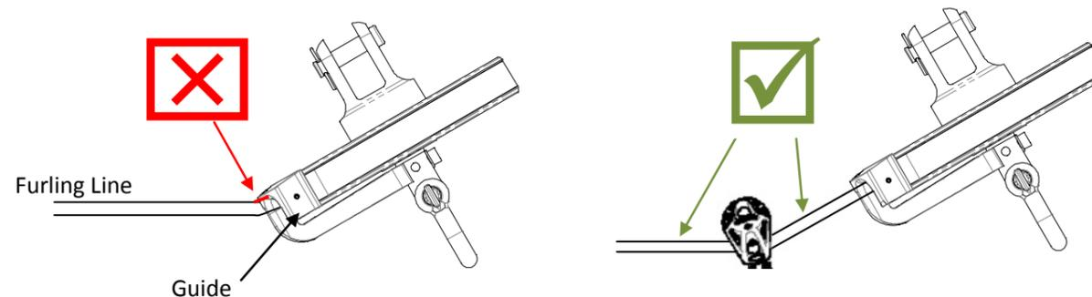
Two Cam cleats can be used to secure the furling line when not in use and keep the sail from unfurling.
