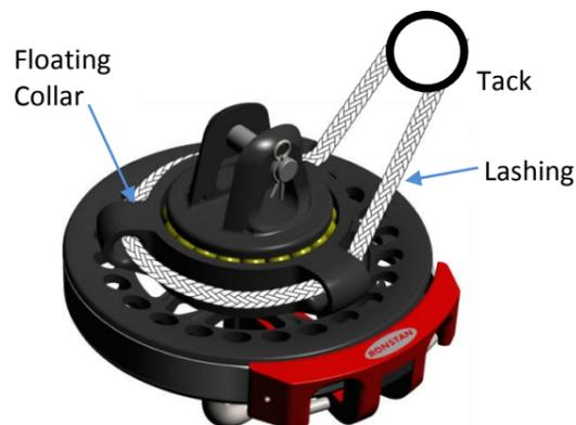
Furling drum rotates, whilst tack remains stationary on “floating” collar. The torsion cable turns the top swivel, furling the sail from the top down.
