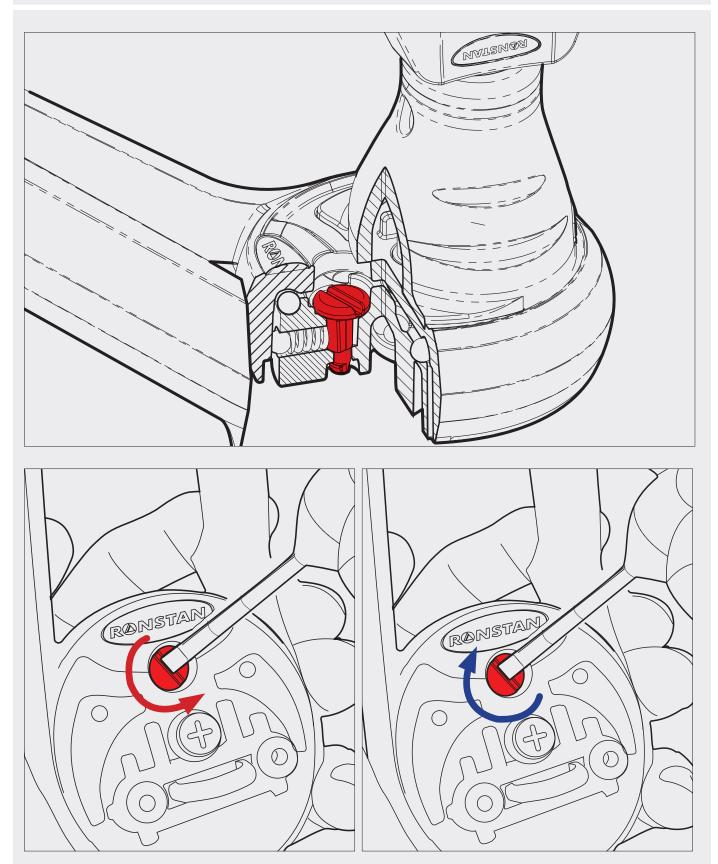
To Disengage - turn switch anti-clockwise. RF6 will swivel freely
