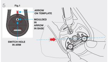
Rotate the arm until the moulded-in arrow on the cleat base appears in the switch hole in the arm (fig.1). With the template still in place on the mounting surface place the RF6 over the template and align the base arrow with the template arrow. While firmly holding down the arm so the base doesn't rotate, turn the arm clockwise until the first mounting hole appears in the switch hole. Fit the first M5(3/16") or 8G mounting screw.
