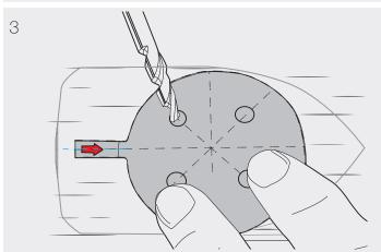
Align the arrow on template with the boat's centre line, pointing forward (toward the bow). This configuration will give equal rotation of the arm to each side, with the arm toward the rear (stern) of the boat.
