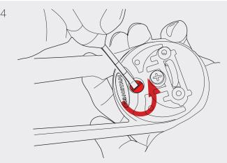
Use a flat head screw driver to turn the red switch counter clockwise until the arm swivels freely.
