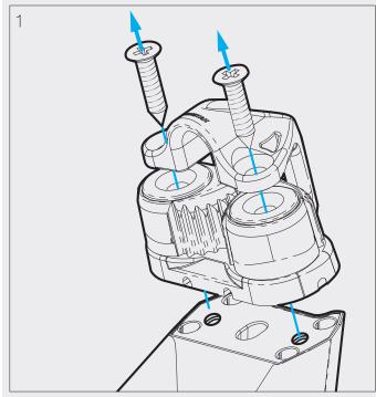
Use a Phillips head driver to remove the cam cleat from the swivel arm. Note keep the 8G screws.
