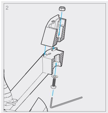
Place supplied M5 nut into cleat riser. Use Allen key to drive cap screw, washer and nut together. Ensure the riser is fitted firmly to the arm.
