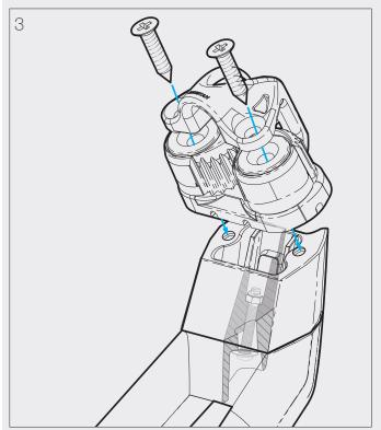
Use a Phillips head to drive the camcleat screws into the pre-drilled holes in the riser.
