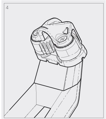
Completed RF6 with cleat riser fitted.
