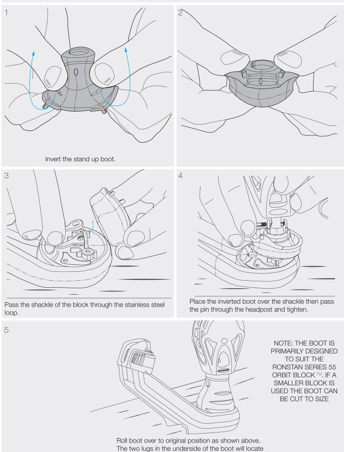
into the holes in the top of the base.
