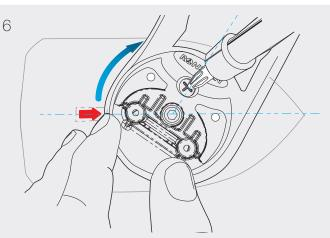
Rotate the arm to locate the other three pre-drilled holes and drive screws into them. There will be two holes either side of the stopper, ensure the arrow on the base remains aligned with the arrow on the template.
