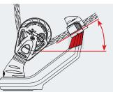
Higher cleating angle with cleat riser fitted to arm
