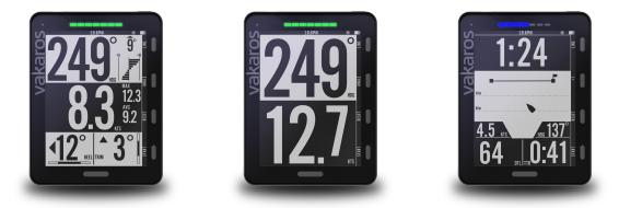
Pressing the home button at the bottom of the Atlas will cycle through all of the different screens currently set up on your Atlas. Each screen is populated by widgets, which display different kinds of data. A few of the default screens that ship with the Atlas 2 are shown above. Using Vakaros Connect, you can add screens and change the existing ones to best suit your needs.
