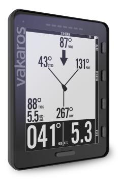
To set up shift tracking on the Atlas, press the ANGLE button to bring up the ANGLE Menu. There are two options for setting port and starboard reference angles, an automatic method and a manual method:
