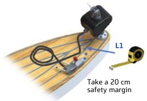
**4** Cut the electric wire ( $L$ ) at the ( $L_1$ ) distance previously measured (+ 20 cm safety margin)
