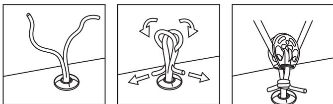
Drill a hole for the TDP. Clean the installation area with acetone to remove dust and grease. Apply Sikaflex 291i or other adhesive to make the installation watertight. Apply pressure to the product to secure it to the installation area. Wait 24 hours before putting any load on the product.
