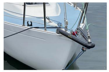
**On-Deck** – Anodized aluminium U-brackets can be bolted through the deck, close to the outboard edge
