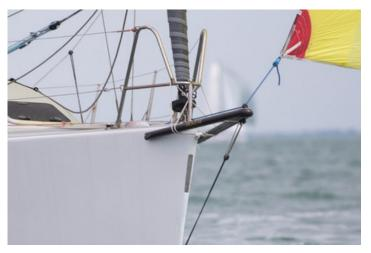
**Through Hull** – The neatest and best solution but does require bonding a glass fibre tube through the bow
