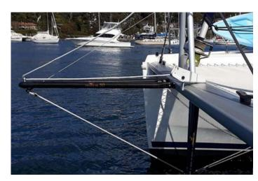
**Catamaran Cross Beam** – Cat Brackets (for the AS40 and AS50 versions only) are bolted on the forward face of the cross beam. Used in conjunction with a dolphin striker
