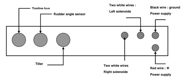
The GYROPILOT 2 **CRP** computer is designed to drive the solenoids of an hydraulic system; This hydraulic system is generally mounted on big boat.
