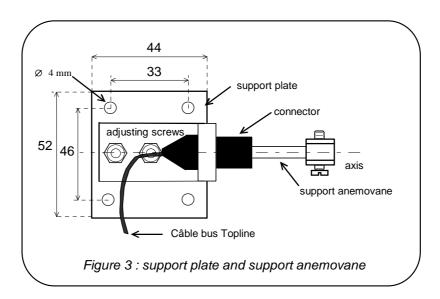
The support plate and the support are assembled using two adjusting screws. At the end of the installation, if the stem of the masthead unit does not perfectly follow the axis of the boat, you can loosen the two nuts in order to align the stem. The plate support must be installed on a horizontal, clean, smooth and flat plane. You will attach the plate using four Ø4 screws (not provided) so that the stem of the wind vane is in line with the axis of the boat.
