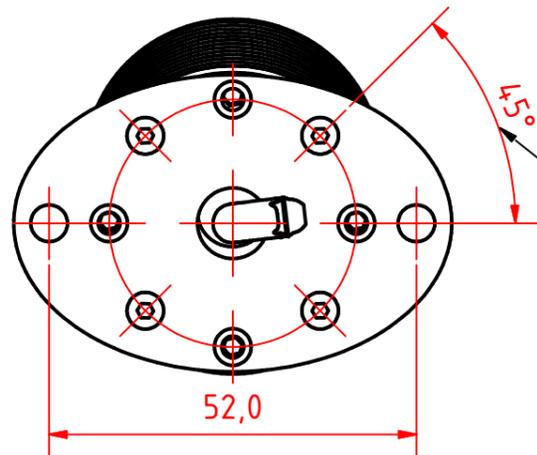
The 10° wedge can be reoriented in relationship to the base plate in 90° Intervals
