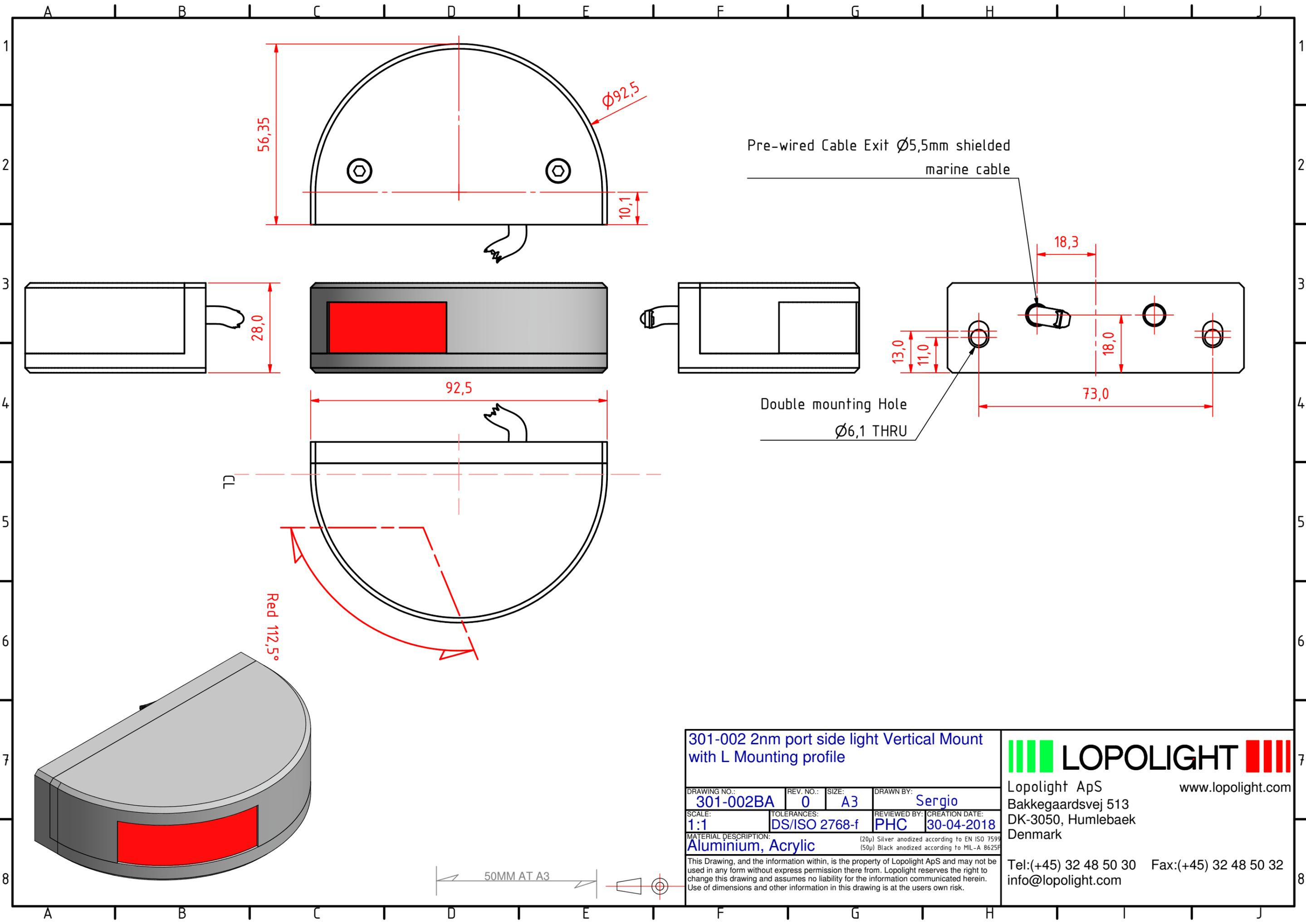
Pre-wired Cable Exit  $\varnothing$ 5,5mm shielded marine cable
