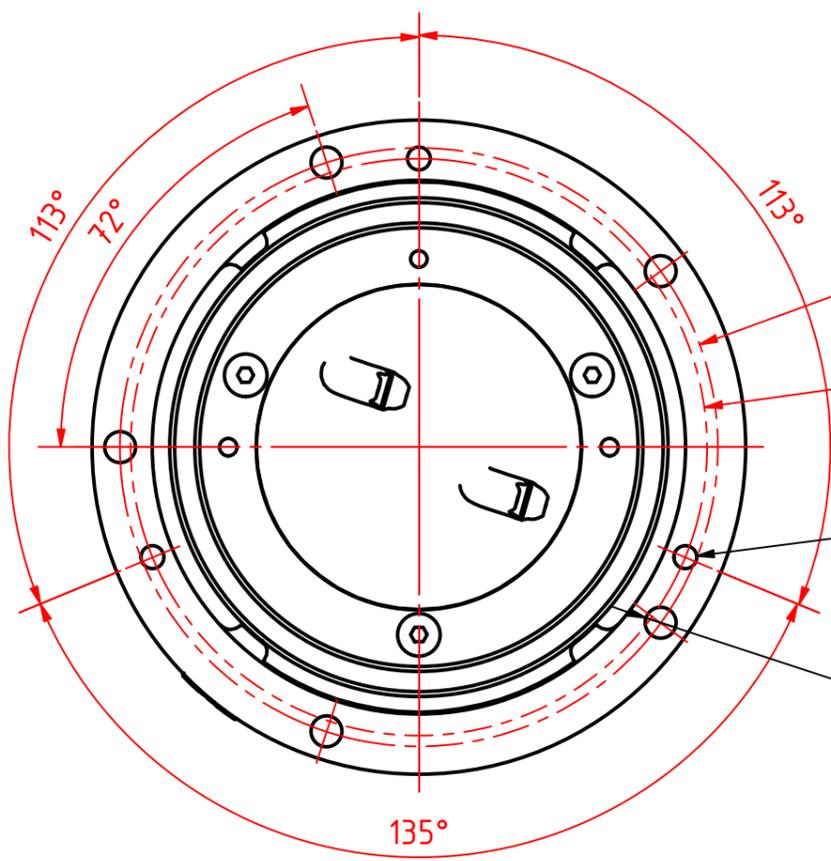
Mounting holes (Mount from underside)
