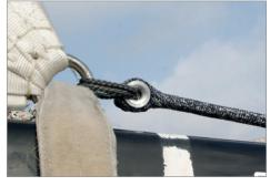
The LOOP<sup>®</sup> Connector on for an outhaul system
