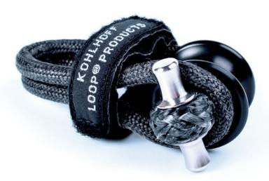
KOHLHOFF LOOP<sup>®</sup> Connectors are lightweight shackles made of a standard Gottifredi Maffioli, Compact Braid loop reinforced by a hard anodized aluminium thimble that provides an exceptional strength-to-weight ratio. This high tech Compact Braid is very strong, light, and waterproof with outstanding abrasion resistance and very low stretch. KOHLHOFF LOOP<sup>®</sup> Connectors can be spliced into outhauls, sheets or halyards to replace standard shackles.
