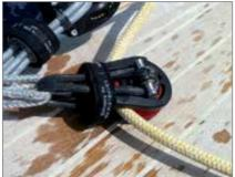
LOOP® Block 60NB as a Code Zero Block on a SWAN 60.
