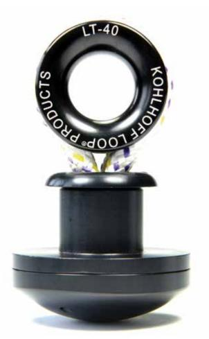
KOHLHOFF LOOP® Padeyes are through-deck fittings made of hard anodised aluminium. Both parts are screwed together to provide easy adjustment for different deck thicknesses. They are all fully water tight with an Acetal cover encapsulating the dogbone and loop on the underside of the fitting. KOHLHOFF LOOP® Padeyes come in black as standard but are also available in silver on request.
