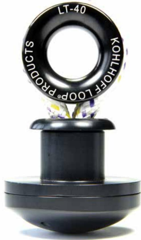
KOHLHOFF LOOP® Padeyes are through-deck fittings made of hard anodised aluminium. Both parts are screwed together to provide easy adjustment for different deck thicknesses. They are all fully water tight with an Acetal cover encapsulating the dogbone and loop on the underside of the fitting. KOHLHOFF LOOP® Padeyes come in black as standard but are also available in silver on request. The Dyneema® loop is NOT supplied as standard and custom loops are also available on request.
