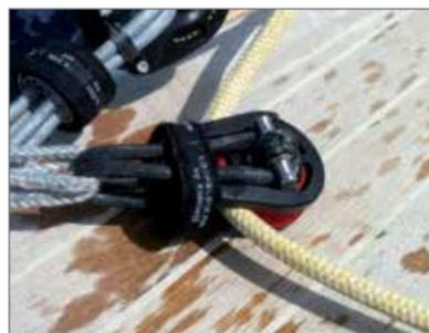
LOOP® Block 60NB as a Code Zero Block on a SWAN 60.
