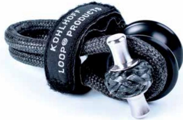
KOHLHOFF LOOP® Connectors are lightweight shackles made of a standard Gottifredi Maffioli, Compact Braid loop reinforced by a hard anodized aluminium thimble that provides an exceptional strength-to-weight ratio. This high tech Compact Braid is very strong, light, and waterproof with outstanding abrasion resistance and very low stretch. KOHLHOFF LOOP® Connectors can be spliced into outhauls, sheets or halyards to replace standard shackles.
