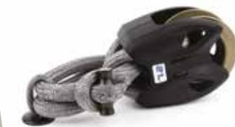
Dyneema SK99 heat-stretched hand-made wined core in a Dyneema cover, sewing finished on aluminium hard anodized I-Bone. Grey, red, blue, yellow, green PU coating. To be used "basket" mounted for short connection 0° or 90°.
