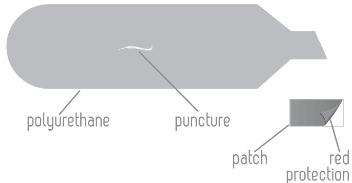
5 Heat up the patch, positioned on the puncture with a hairdryer (around 1 minute) with keeping a distance of 20 cm (between the patch and the tip heating of the hair dryer) until the patch sticks totally on its area (do not hold the patch with fingers during the operation).
