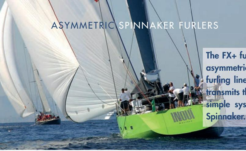
The FX+ furler, fitted with the Fast thimble, allows to furl in the asymmetric Spinnakers from the cockpit by pulling the bottom furling line. The anti-twist rope rotates up to the top and then transmits the rotation from the head to the tack of sail. With this simple system it is possible to use your existing asymmetric Spinnaker.
