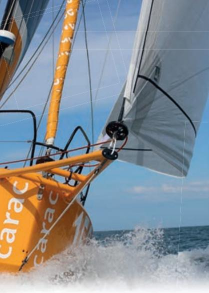
Further to constructive technical exchanges with ocean racers, Facnor has developed a sophisticated range of Gennaker/Code Zero furlers : the FX+. A true evolution : light, easy to fit and aesthetic. Fitted on request with a ratchet device securing the furling, locking both clockwise and anti-clockwise (Facnor patent).
