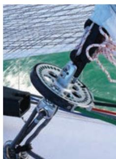
a Staysail can be fitted on a FX+ furler so that a stormsail can be used according to the weather conditions. In this configuration, we recommend to install a 2-to-1 block (halyard better tighten and less tension
