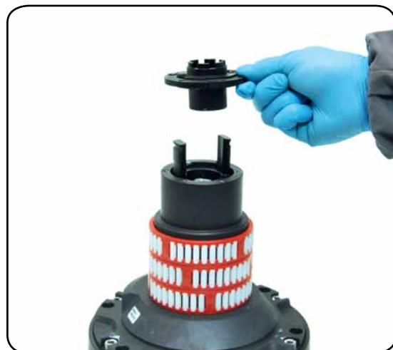
6. Remove the stripper arm housing n°21
