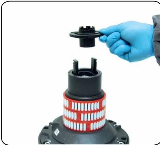
6. Remove the stripper arm housing n°21
