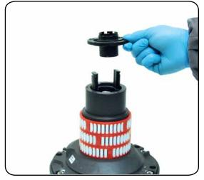
6. Remove the stripper arm housing n°21
