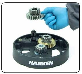
13. Remove the idler and pinion  $n^{\circ}14$
