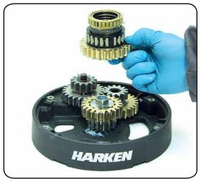
11. Remove the gear n°33, pawls carrier n°32, the bearings n°34 and 36 and the pin n°35. Important: washer n°7 may remain inside the drum support!
