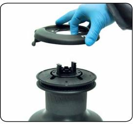
4. Remove the self-tailing arm n°26 by rotating and lifting it.
