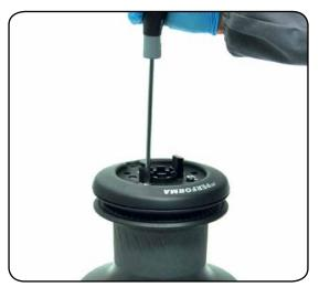
3. Unscrew the three screws n°27 (~4Nm/35 in-lb)
