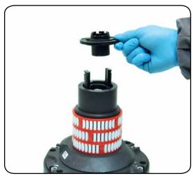
6. Remove the stripper arm housing n°21
